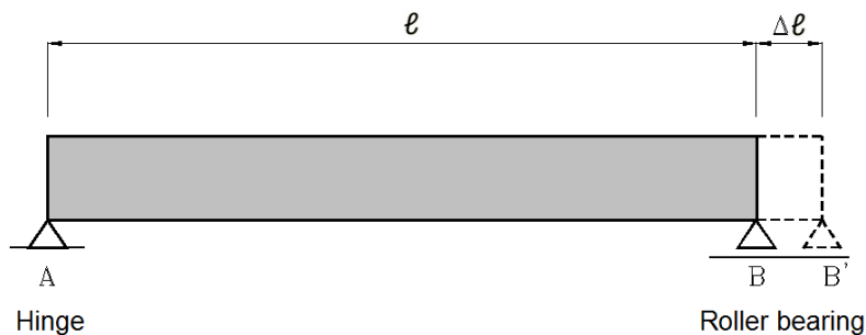
Figure 17-2 Increase in the length of a beam due to a total rise in temperature
