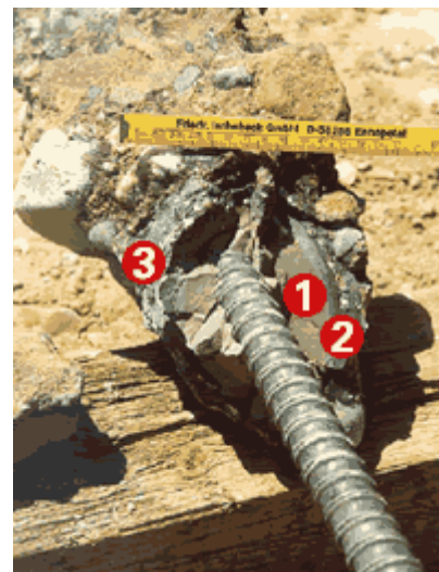
Figure 39-9 Installation of self-drilling grout anchor. ( http://www.ischebeck.de )
