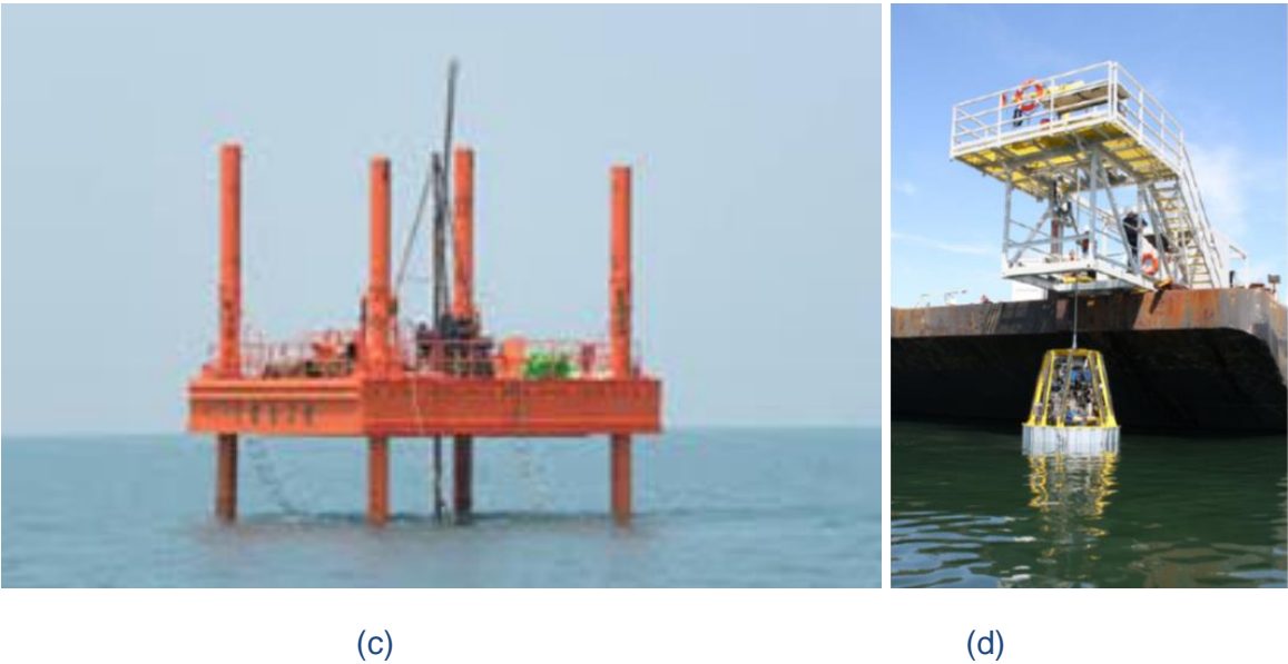
Figure 3.6 (a) Standard CPT rig, (b) Light-weight CPT rig, (c) Jack-up rig (d) sea-bed mounted rig
