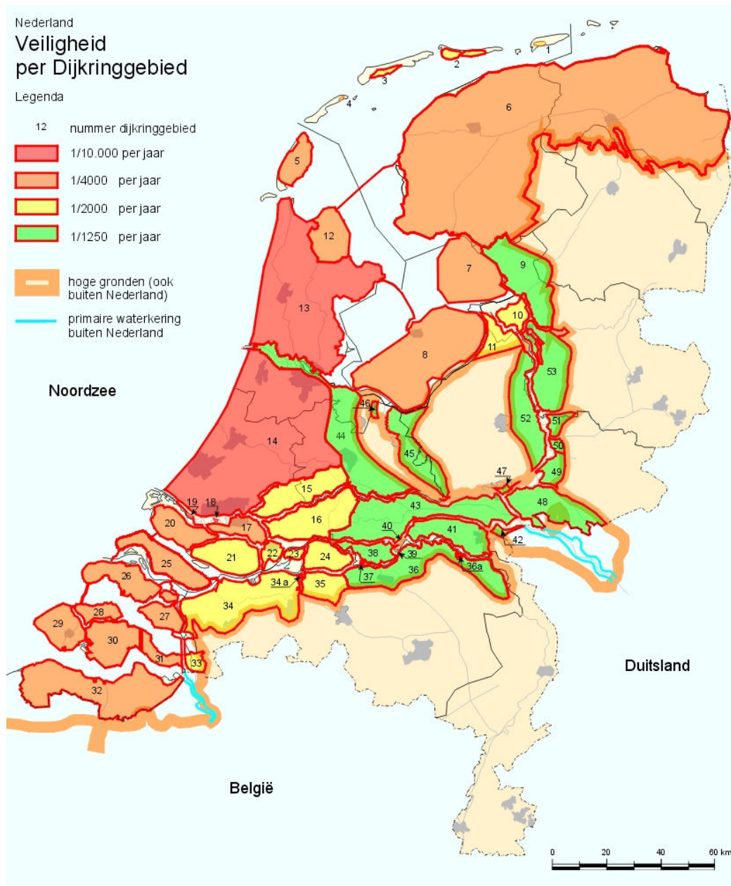
Figure A.3: Dike ring areas with an approximately equal flood risk, but different exceedance probabilities
