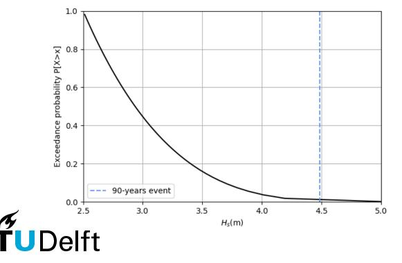
Load: significant wave height (T<sub>R</sub>=90 years)
